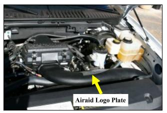
**9.** Double check your work to be certain that all nuts, bolts, and clamps are securely fastened. Fasten the Logo Plate to the intake Tube as shown, using the two Button Head Screws.
