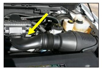
**1.Disconnect The Negative Battery Terminal!** Disconnect intake tube from air filter housing by unsnapping the tube assembly from the housing.
