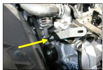
**3.** Remove 13mm nut on power steering reservoir bracket. Install Airaid Modular Intake Tube support bracket, replace nut, and leave slightly loose. (Nut will be tightened after final adjustments.)
